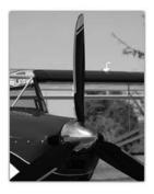
The WhirlWind GA propeller series are ground pitch adjustable aircraft propellers featuring advanced aerodynamic and composite design.
